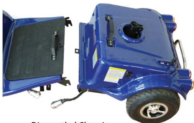
Dismantled Chassis Showing Quick Release Electrical Coupling
